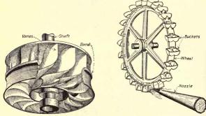
Fig. 289.—Runner of a mixed-flow turbine.
